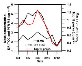
**Figure 2**. Time series profile of total organic matter (TOM) measured using DRI OC/EC and PTR-MS, including the major peaks observed in the mass spectra.
