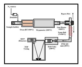
Figure 1. Schematic diagram of the tandem instruments. Included also here are the relevant instrument settings used in this study.
